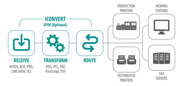
The system communicates with host systems and appears as IPDS devices or LUs. iCONVERT dynamically transforms AFP reports into a variety of other print languages and routes the resulting data to distributed network and production printers, archiving systems, and viewing stations. The SPDE Line Mode::AFPDS module converts AFP formatted line and mixed mode data into fully composed AFPDS for further processing by the AFPDS modules.
