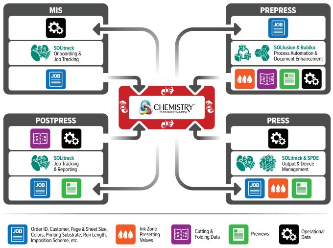
Solimar uses JDF/JMF as one communication method to acquire data that informs workflow processes and share data between applications as needed. The Solimar® Chemistry<sup>™</sup> platform products Rubika®, Solimar® Print Director<sup>™</sup> Enterprise (SPDE), and SOLitrack<sup>™</sup> leverage JDF to automate communication and supply data to tracking elements.
